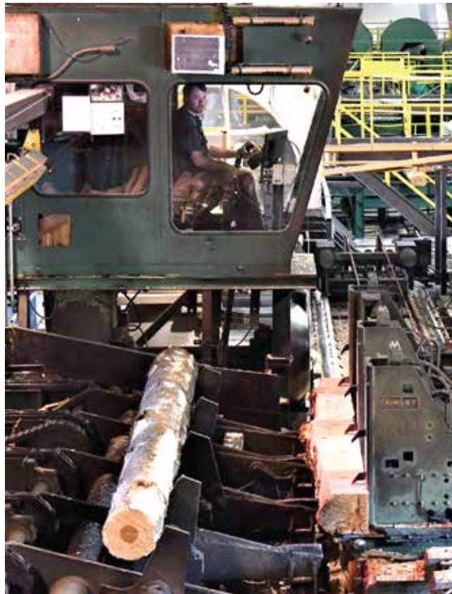
A sawyer at Neiman Enterprise’s Hill City, South Dakota mill squares a log before sawing it into lumber. Computer guided laser lights scan each log to determine how best to saw it, minimizing waste by maximizing the amount of lumber of varying dimensions that can be recovered from each log.
