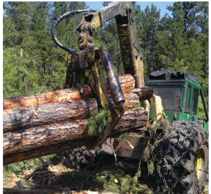
Terrain in much of the Black Hills is gentle enough to permit rubber-tired skidders to transport logs to sites where they are loaded on trucks destined for the area's sawmills. To minimize soil erosion, temporary roads are blanketed with tree limbs and branches that eventually decompose, enriching the soil in which seedlings will regenerate naturally.
