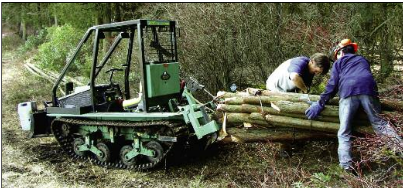
Schaier's crew clear-cuts cedar but subcontractor Vinh Lang uses compact Forcat 2000 skidder to thin young cedar stands on New Jersey's Haines Stewardship Forest. Powered by a 27 HP Kohler engine, the machine's ground pressure is about 2.5 PSI.
