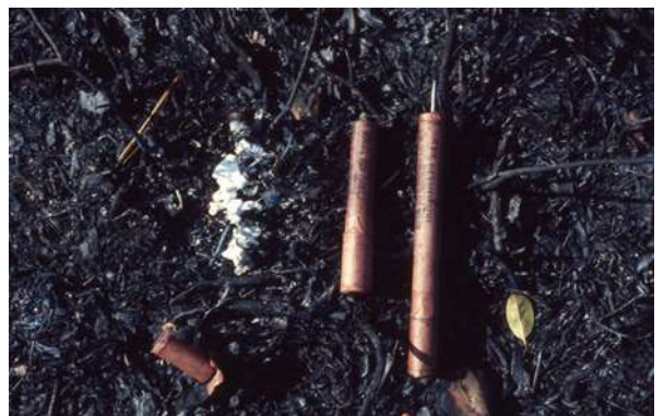
SAMPLES of HIGHWAY FUSEES and CHAR at FIRE ORIGIN
