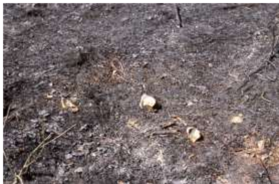
BROKEN INSULATOR at ORIGIN
