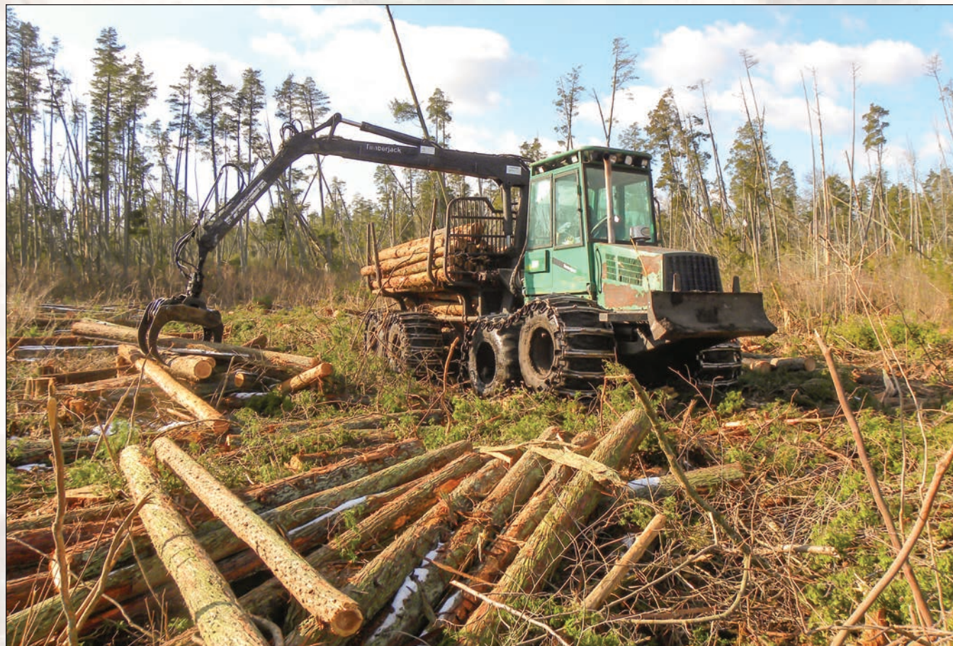
To reduce rutting, Advanced Forestry Solutions keeps Clark tracks on its Timberjack forwarders.
