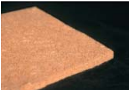
Lab scientists made this inexpensive fiber mat made from juniper. It is capable of filtering many contaminants from water.
